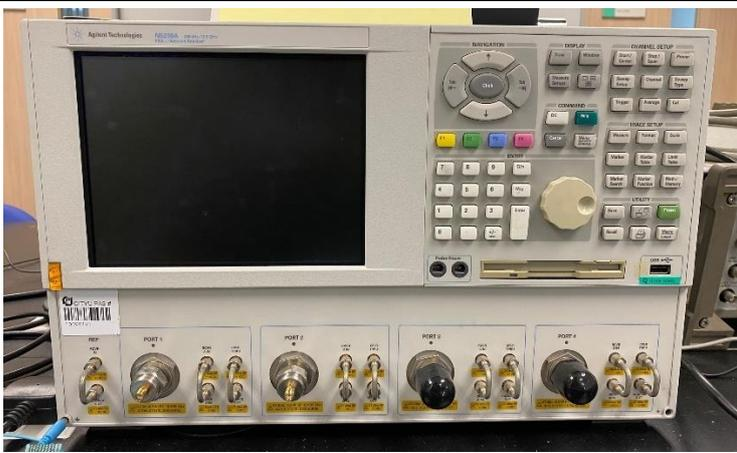
A photograph of an Agilent Technologies N5239A Network Analyzer. The device is a rack-mountable instrument with a large black display screen on the left. To the right of the screen is a control panel featuring a central rotary knob, several function buttons, and a numeric keypad. Below the control panel, there are four main ports labeled PORT 1, PORT 2, PORT 3, and PORT 4, each with multiple connector options. The front panel also includes a power button and various status indicators. |
